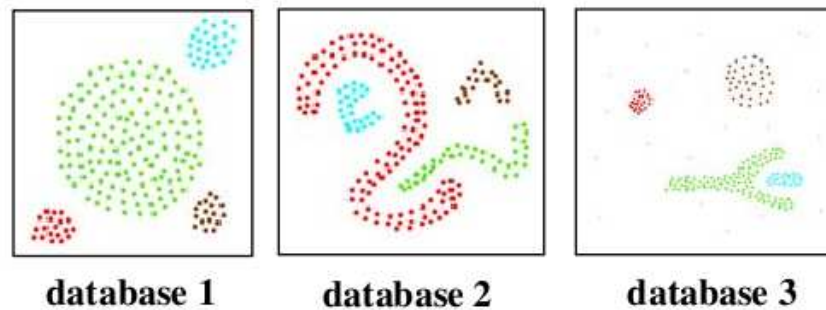
figure 6: Clusterings discovered by DBSCAN
